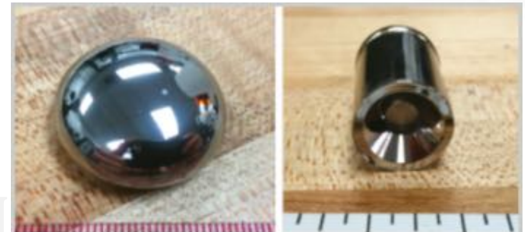
(Left) A 30-g ingot of the BMG \text{Ti}_{40}\text{Zr}_{20}\text{Cu}_5\text{Al}_5\text{Be}_{30} with a measured density of 4.76 \text{ g/cm}^3 after alloying in a plasma arc melter from pure elements. The ingot is fully glassy after melting. (Right) The ingot from the left cast into a 16-mm diameter cup-and-cone insert for latching operations on a proposed spacecraft.
